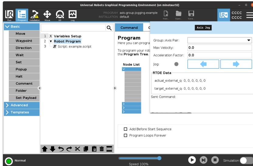
3. Select the desired Axis to jog, and enter the preferred parameters specific to the Axis
