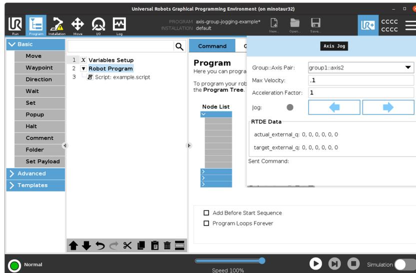
4. Jog the given Axis by holding down either the <- or -> button
