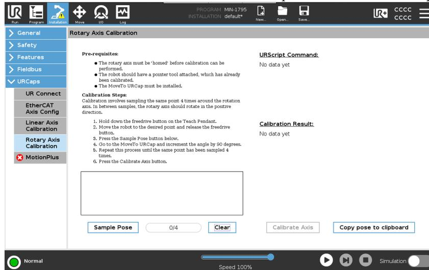
See below images for reference on how to use the MoveTo URCap to increment the rotary axis:
