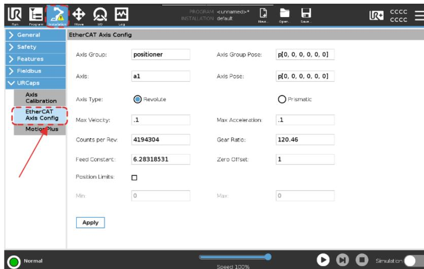
2. Changes made to the axis configuration will persist in the DataModel. Notice how a change in the Max Velocity adds an asterisk to the installation indicating that changes have been made.
