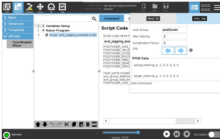
4. Jog the first Axis of the given Axis Group by holding down either the <- or -> button
